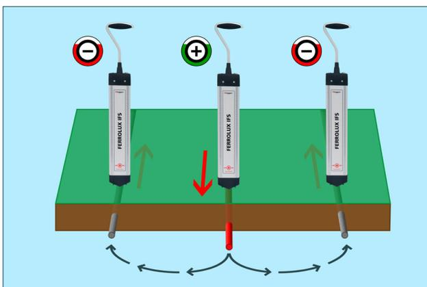
If there are several lines (cables, pipes) located next to each other, it is often difficult to determine which the correct one is. Sometimes the signal from the generator can flow through both lines, but the signal in the lines may be flowing in different directions. With the SignalSelect function, the generator applies a signal that contains directional information. When the device is positioned over the correct cable, a "+" symbol is displayed to facilitate precise identification.
